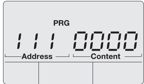
Fig. example of the display; connection for the auxiliary measurement, address 111 with the content 0000 (=2w1n).
