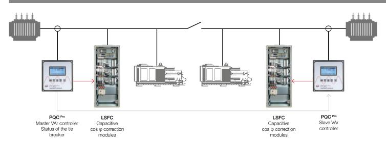
FRAKO modular power factor correction units, combined with the unbeatable versatility of the PQC  $^{\text{Pro}}$ , make it possible to accomplish a wide variety of  $\cos \phi$  correction duties with optimum results. Whether inductive or capacitive corrective power is required, the watchword is always "Connect – ready – run".
